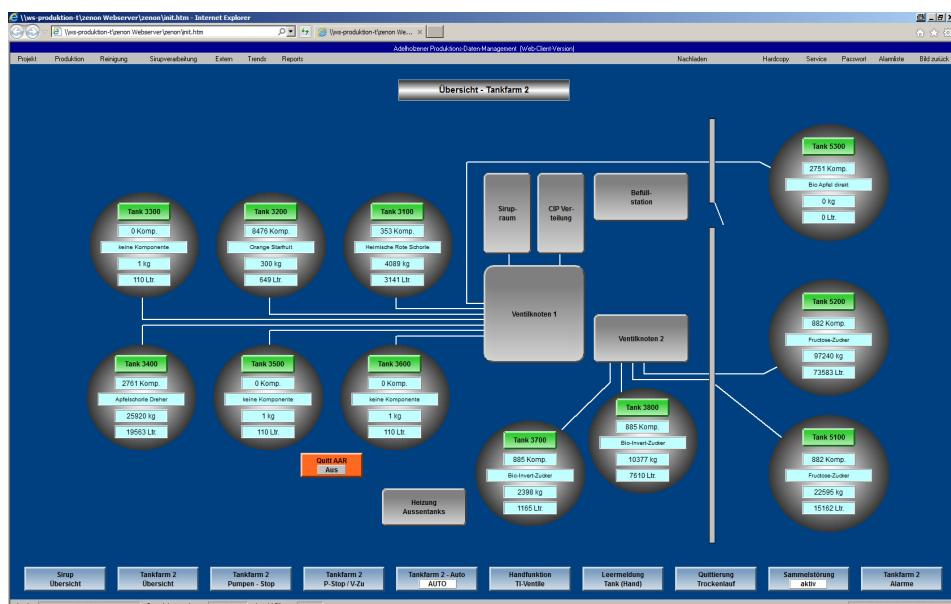
The visualization of the tank storage is part of the production data management and shows, for example, the respective fill levels of the tanks.
