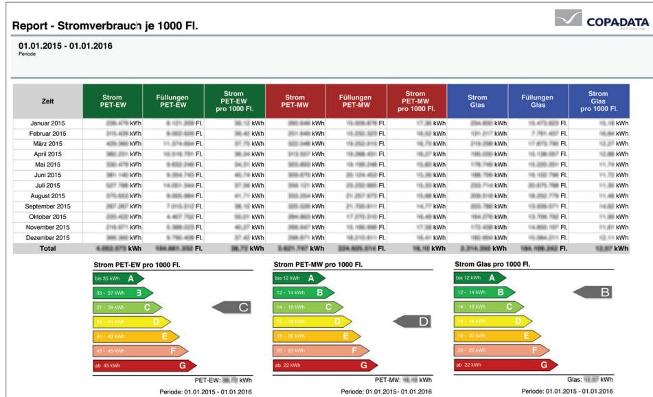
*Reporting with the zenon Analyzer: In this report, Adelholzener is showing the power consumption per 1,000 liters of filled bottles during the year. The energy consumption is also divided into energy efficiency classes for PET reusable bottles, PET single-use bottles and glass bottles.*
