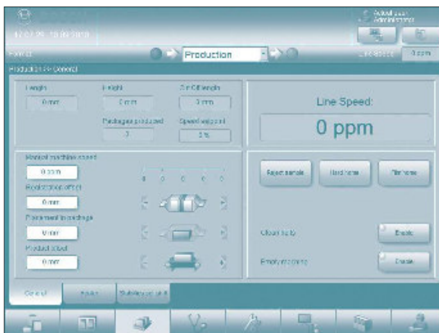
The production display informs the user at Bosch Packaging Systems about all relevant parameters. The upper screen section shows information on the product dimensions (left) as well as machine speed (right). The user can use each input field (center of screen, left) to make offset corrections to the product or foil positioning.
