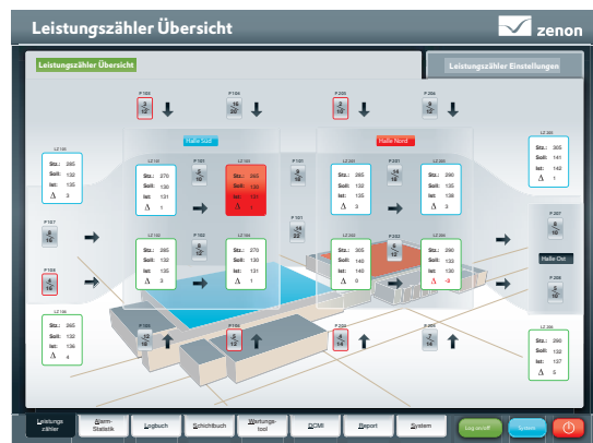
Display of production states with the help of traffic light colors
