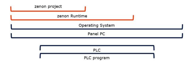
Figure 1: Components layers of a typical PLC and HMI application
