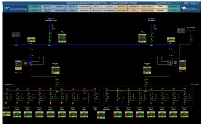
A single line diagram with statuses, control option and basic data measuring with ALC function
