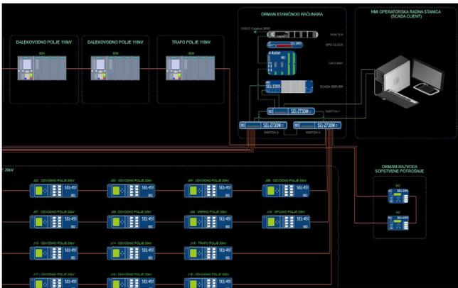
Communication block schematic showing equipment status and communication links at Šipovo Substation
