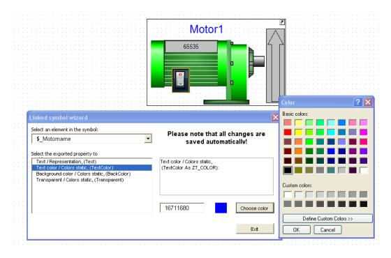
Figure 10: With the help of the assistant, any desired symbol property - for example the color (as shown in the picture) - can be changed.
