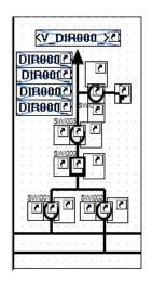
Figure 3: Branch with many linked symbols, which can be changed from a central location.
