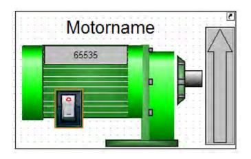
Figure 8: Symbol on the screen, with allocation of variables.
