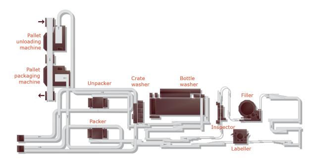
Figure 2: The packaging line, the object for the implementation of an Equipment Performance System
