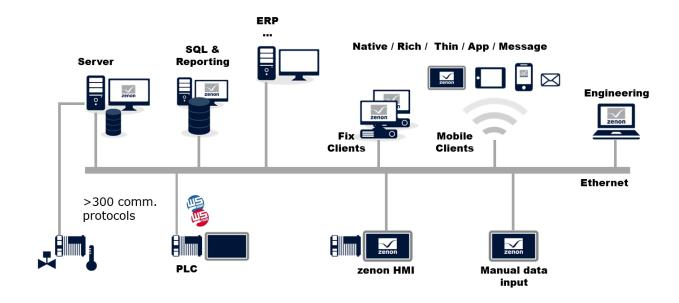
Figure 9: Architecture of an EPS, integrated from production area to ERP level
