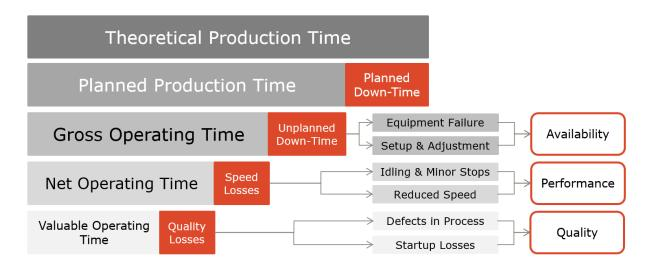
Figure 1: OEE is not just an indicator; it brings focus on potential improvements.
