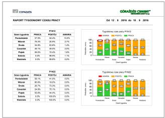
A weekly report shows working time, standby time, and standby time because of alarms.
