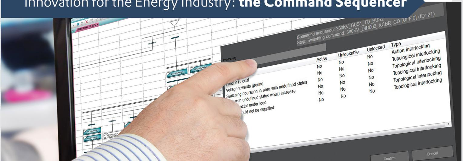
The Command Sequencer simplifies project configuration and setting command sequences massively. The operator can, intuitively and without programming knowledge, compile sequences of commands, test these and apply them. The same also applies for changes in the command sequences. Project configuration is carried out in a graphic editor in Runtime, either by means of selection and compilation of the individual steps, or by means of teaching. With teaching, the system
