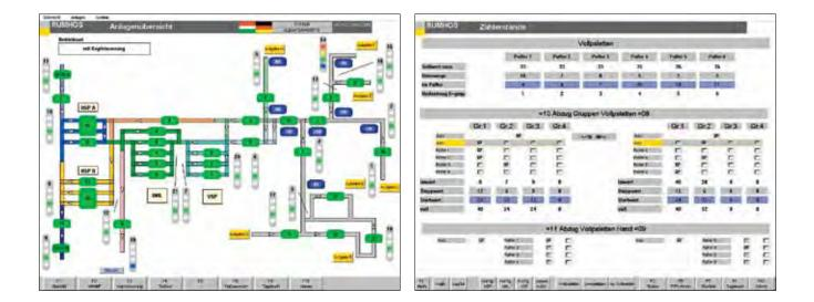
and detects weak points in the facility. Additionally, the sophisticated monitor administration helps to make the Maintenance team's work a lot easier: the process pictures are split between two monitors. This way, the user can have an overview picture displayed on one monitor and a detailed picture on the other monitor.
